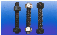
Actual corrosion tests. Left: Xylan bolt - moderate coating and oxidation damage. Nuts not frozen. Center: Cadmium plated bolt - total coating failure. Severely corroded. Right: Plain steel bolt - bolt utterly destroyed. Would fail in service. Photo: Whitford
